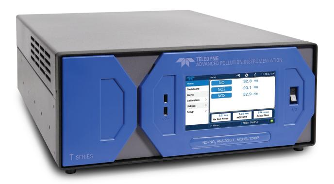
The Model T200P provides measurements of NO,  $NO_x$  and  $NO_2$  using our T200 Chemiluminescence analyzer combined with a patented high efficiency Blue Light Converter (BLC). The BLC, also known as photolytic converter, provides a very specific conversion of  $NO_2$  with conversion efficiency similar to molybdenum.\*
