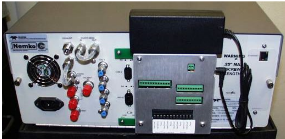
Figure 2-9. Calibrator Rear Panel Valve Driver Installed (with PSM connected to JP1)
