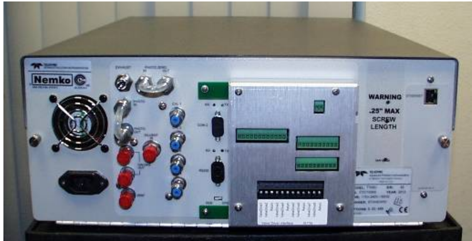
Figure 2-10. Calibrator Rear Panel Valve Driver Installed (without PSM)
