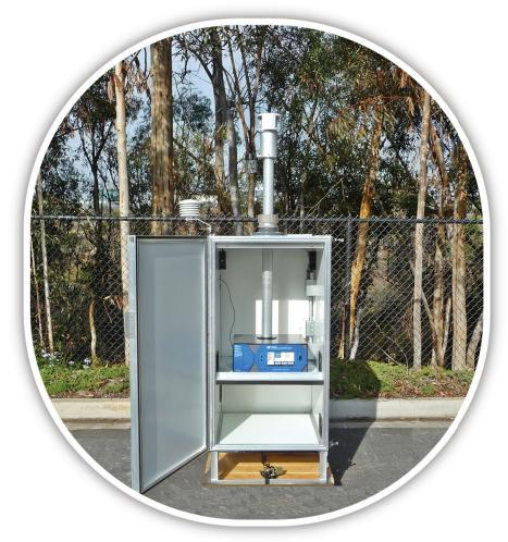
Teledyne API offers an Outdoor Enclosure option for our Model T640 PM instrument. Its rugged design is ideal for long or short term monitoring projects in outdoor environments where other weather protection is unavailable. The enclosure has internal, thermostat-controlled fan ventilation and can operate in ambient conditions ranging from -20°C to 50°C.
