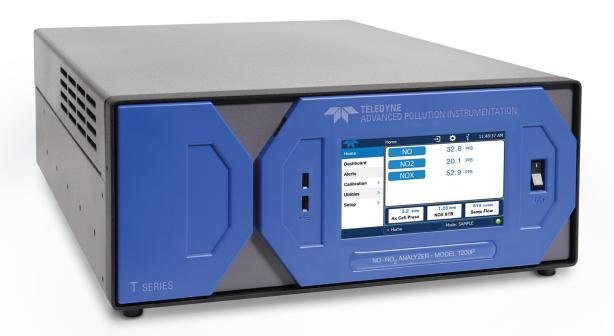
The Model T200P provides measurements of NO,  $NO_x$  and  $NO_2$  using our T200 Chemiluminescence analyzer combined with a patented high efficiency Blue Light Converter (BLC), also known as photolytic converter. The BLC provides a very specific conversion of  $NO_2$  with conversion efficiency similar to molybdenum but without the same interferences.\* The T200P is ideal for ambient and roadside monitoring.
