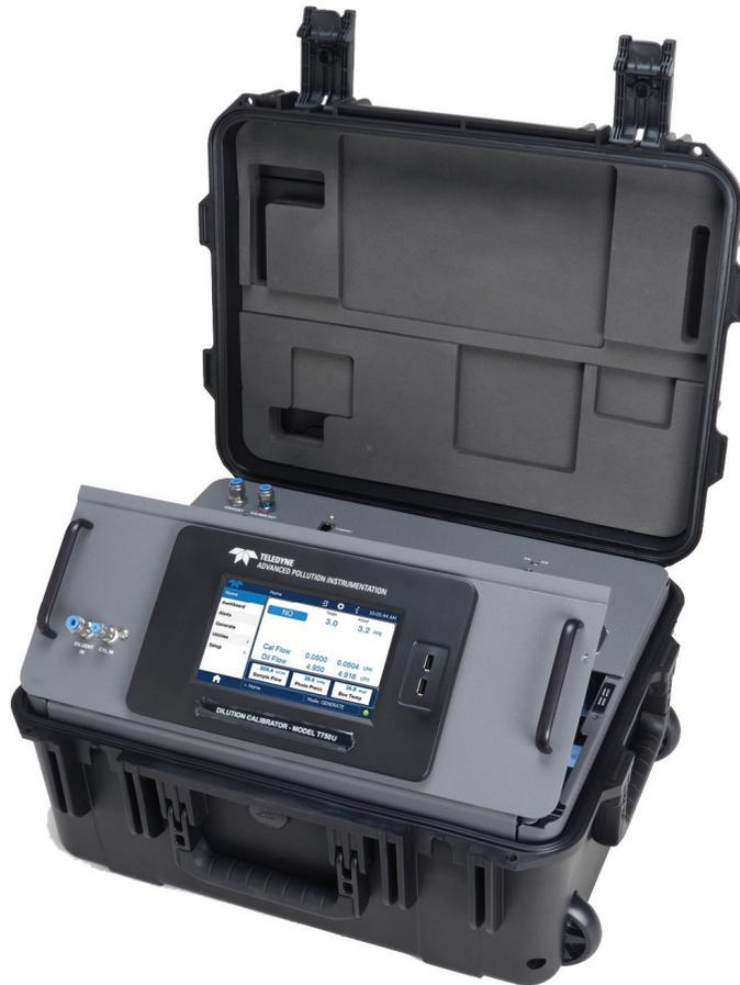
A portable, microprocessor based calibrator for precision gas analyzers, the Model T750U combines highly accurate mass flow controllers and compressed sources of standard gases to provide multipoint span and zero calibrations. The T750U includes two operating modes: a high range with similar performance to the Model T750 instrument with ozone generator, and a low range which includes a "fractional mode" for producing accurate and stable O<sub>3</sub> and NO<sub>2</sub> levels down to 3 ppb.
