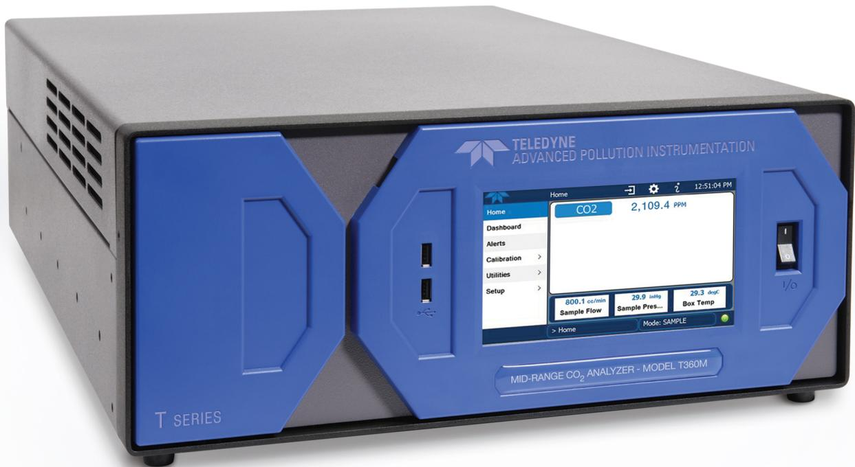
Using a gas filter correlation wheel, the Model T360M Mid-Range CO<sub>2</sub> Analyzer measures carbon dioxide by comparing infrared energy absorbed by a sample to that absorbed by a reference gas according to the Beer-Lambert law. This design produces excellent zero and span stability and high signal to noise ratio, allowing excellent performance over a wide concentration range, making this instrument an ideal choice for CO<sub>2</sub> reporting requirements associated with dilution CEMS.
