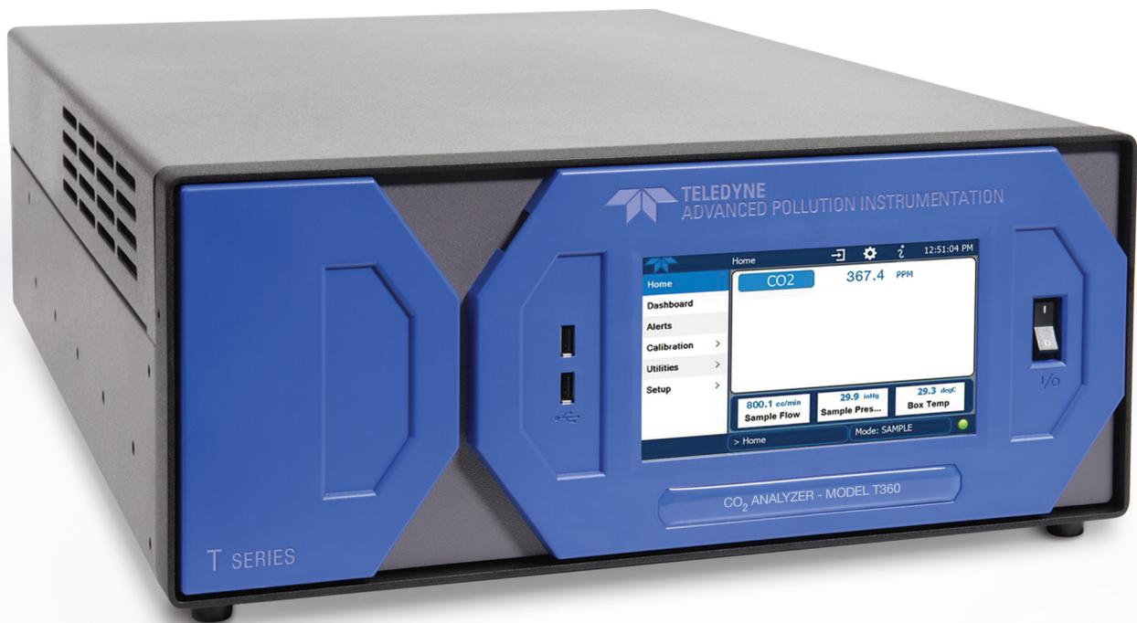
Using a gas filter correlation wheel, the Model T360 CO<sub>2</sub> analyzer measures carbon dioxide by comparing infrared energy absorbed by a sample to that absorbed by a reference gas according to the Beer-Lambert law.
