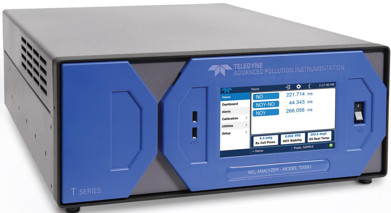
The Model T200U NO<sub>y</sub> analyzer has been developed and refined specifically to address the challenges of NO<sub>y</sub> monitoring, for example in the US NCore network. It uses the proven Chemiluminescence principle and is coupled with a remote NO<sub>y</sub> converter via umbilical to allow measurements with a lower detectable limit of 50 ppt.
