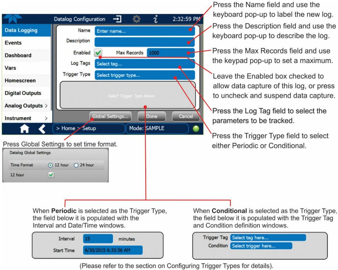
Press the Name field and use the keyboard pop-up to label the new log.
