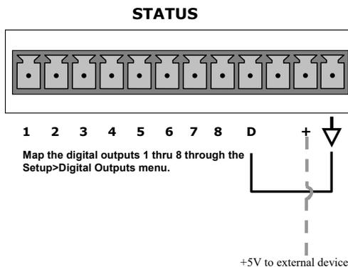
**Figure 2-6. Status Output Connector for Digital Outputs**
