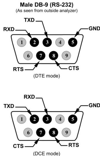
**Figure 2-9. Rear Panel Connector Pin-Outs for RS-232 Mode**
