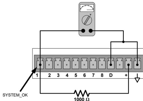
**Figure 5-12. Typical Set Up of Status Output Test**
