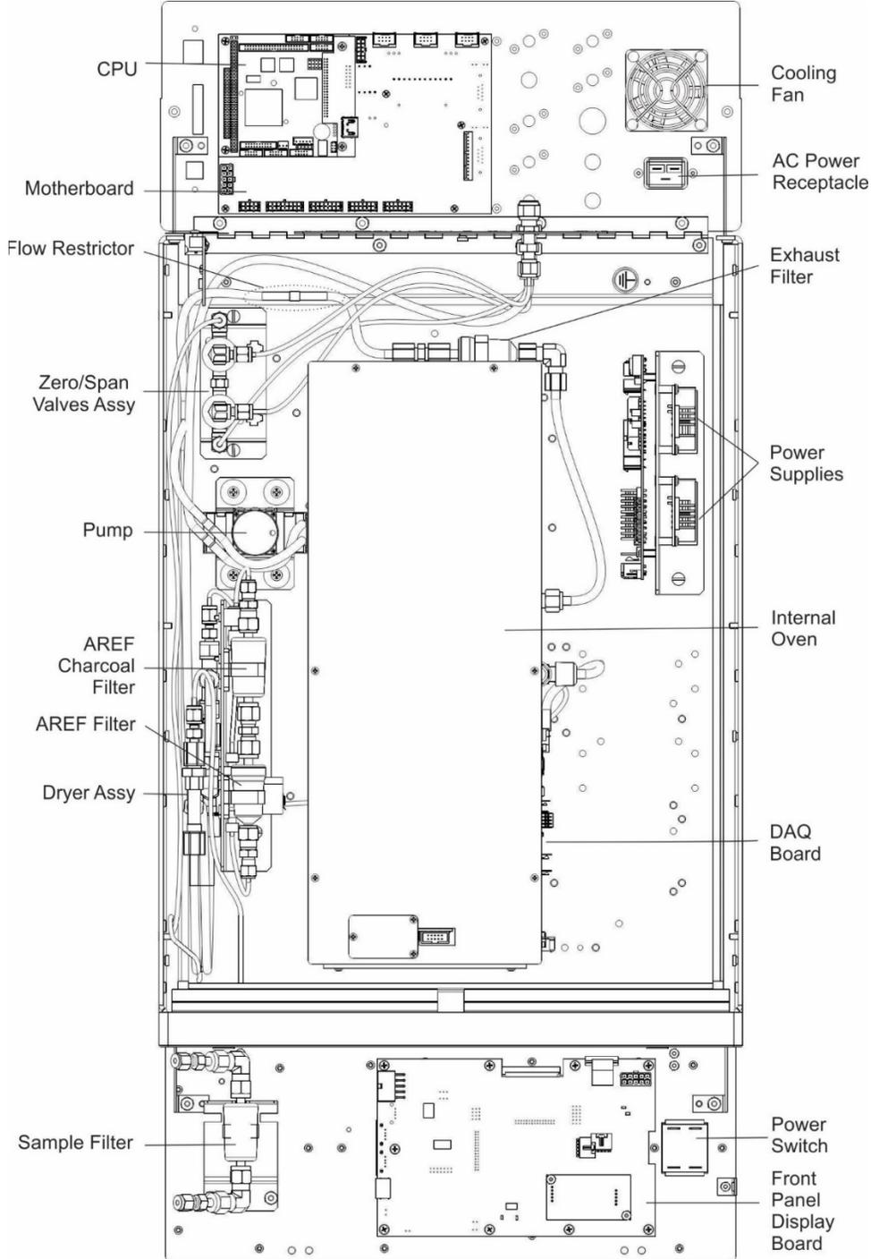
**Figure 2-3. Internal Chassis Layout**
