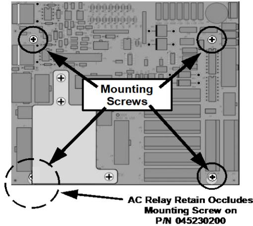
**Figure 5-14. Relay PCA Mounting Screw Locations**
