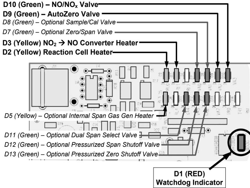
**Figure 5-9. Relay PCA Status LEDs Used for Troubleshooting**
