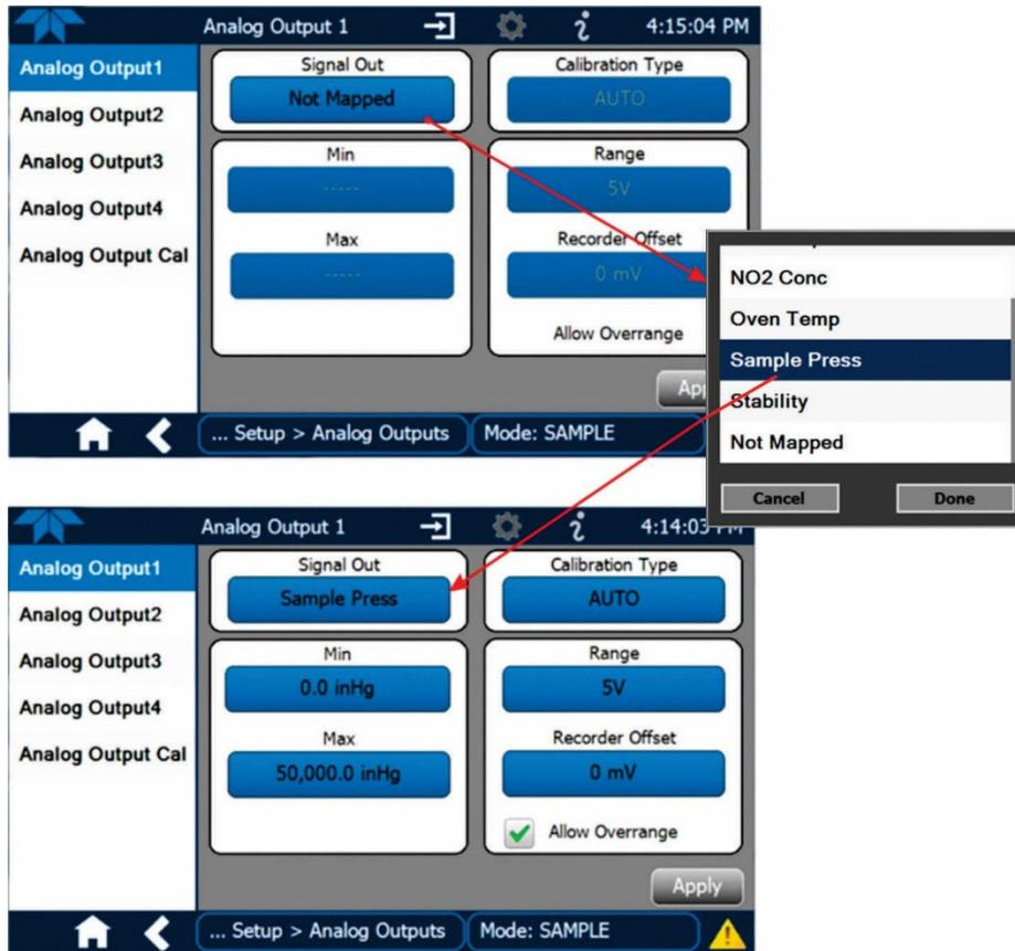
**Figure 2-39. Analog Output Configuration Example**
