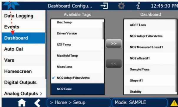
Figure 2-36. Dashboard Display and Configuration
