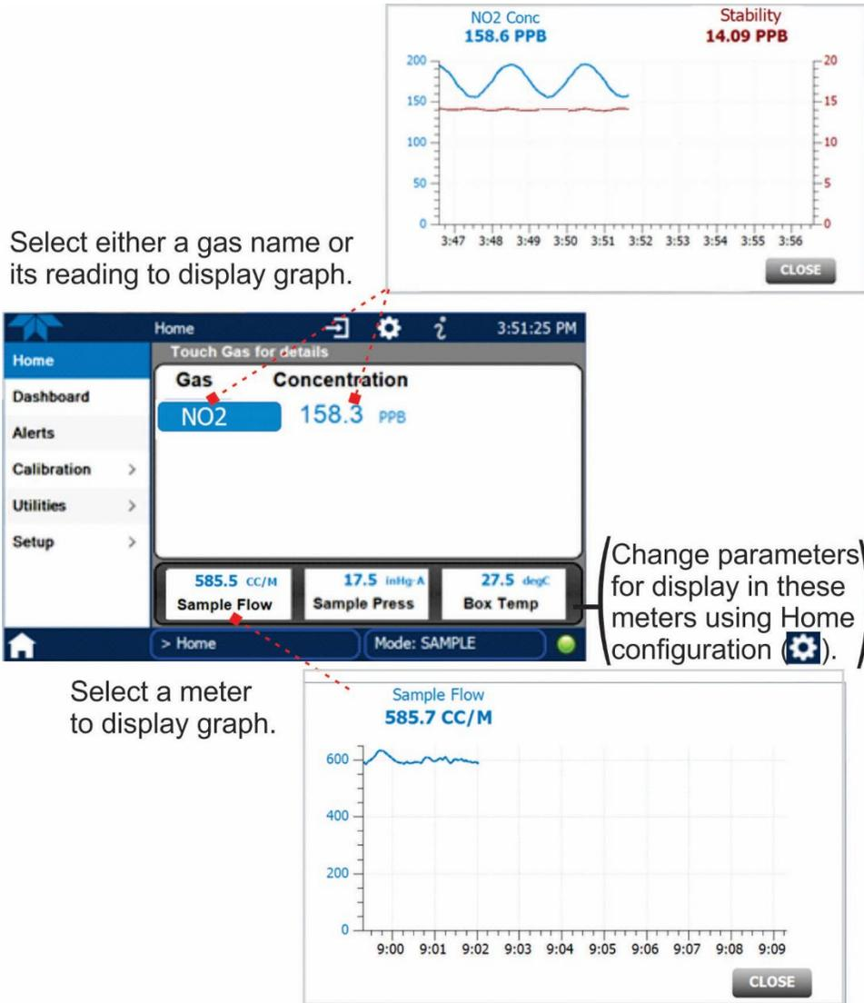
Figure 2-21. Concentration and Stability Graph (top) and Meter Graph (bottom)
