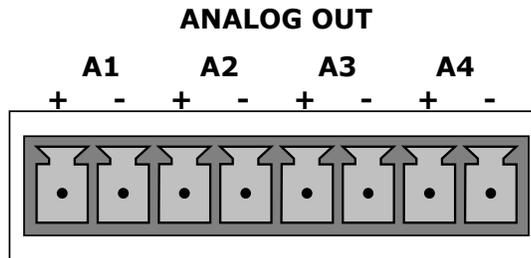
**Figure 2-4. Analog Output Connector**
