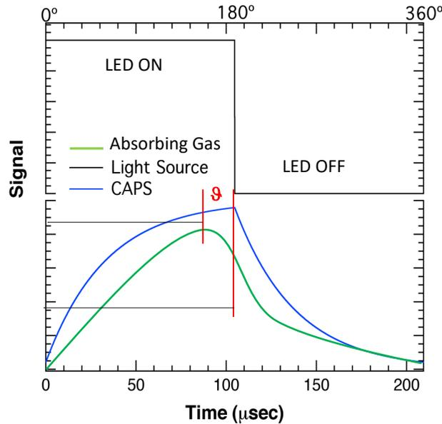
**Figure 6-2. Phase Shift Representation of Increased Concentration of NO<sub>2</sub>**
