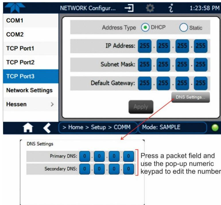
**Figure 2-45. Communications Configuration, Network Settings**
