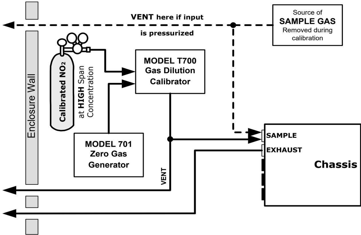
**Figure 2-13. Gas Line Connections from Calibrator – Basic Configuration**
