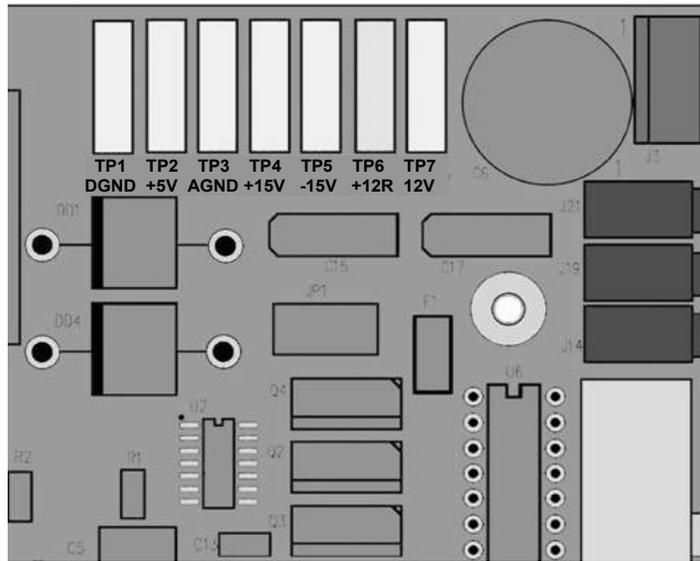
**Figure 5-10. Location of DC Power Test Points on Relay PCA**
