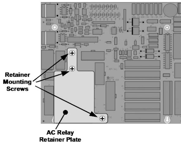
**Figure 5-13. Relay PCA with AC Relay Retainer In Place**
