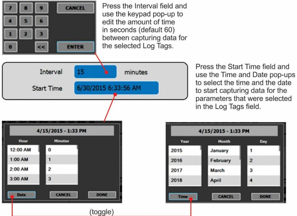
Press the Interval field and use the keypad pop-up to edit the amount of time in seconds (default 60) between capturing data for the selected Log Tags.
