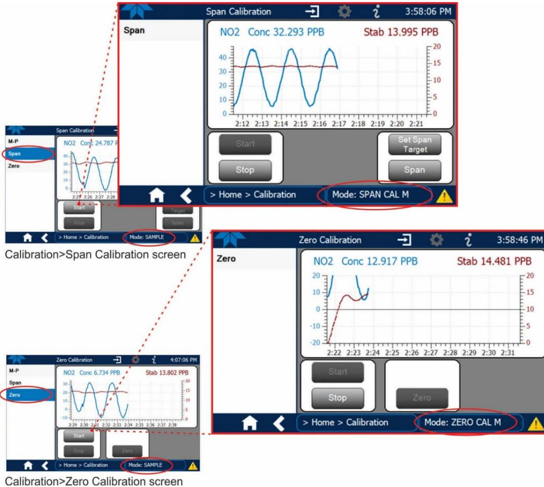
**Figure 4-2. Zero and Span Calibration Screens**
