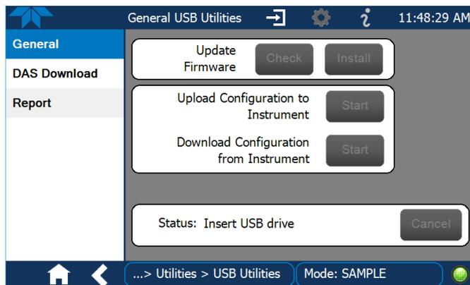
**Figure 2-46. Configuration Transfer**
