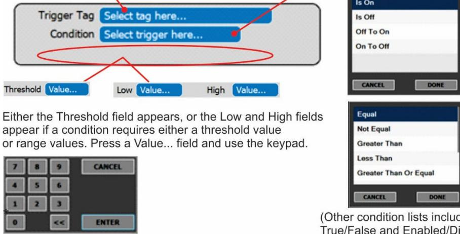
Either the Threshold field appears, or the Low and High fields appear if a condition requires either a threshold value or range values. Press a Value... field and use the keypad.
