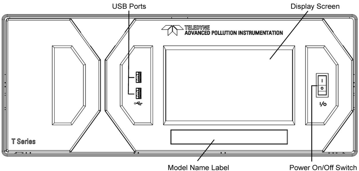
**Figure 2-3. Front Panel Layout**
