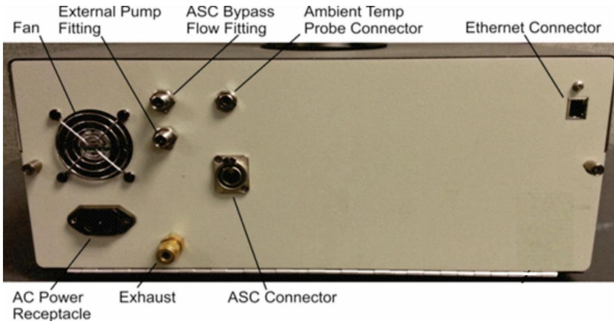
Figure 2-5. T640 with 640x Option Rear Panel
