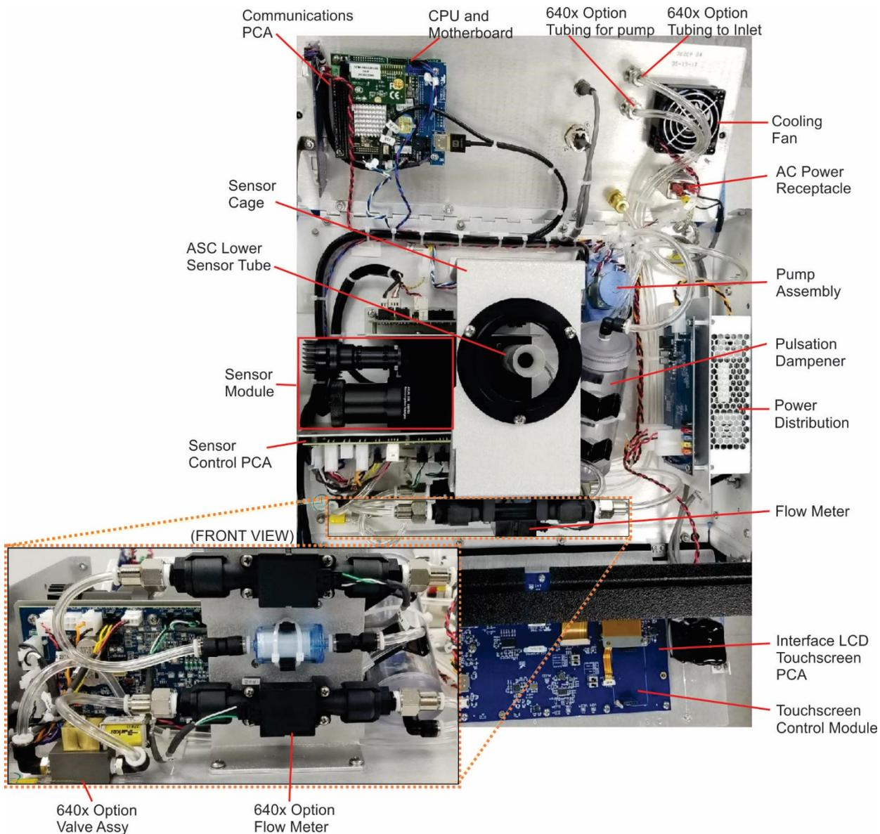
Figure 2-6. T640 Internal Layout, with 640x Option Components
