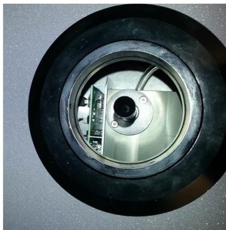
Figure 2-7. Top View of Inlet Nozzle
