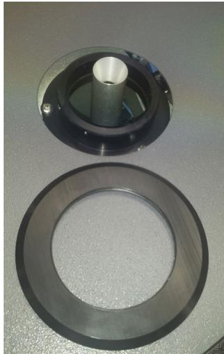
**Figure 2-9. Collar for Lower Flange**
