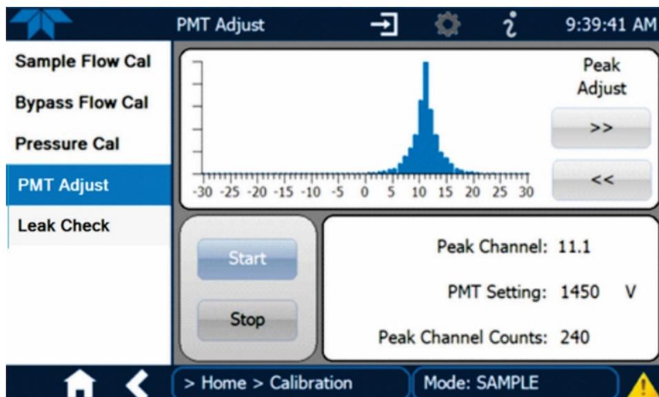
Figure 4-5. PMT Adjustment Menu
