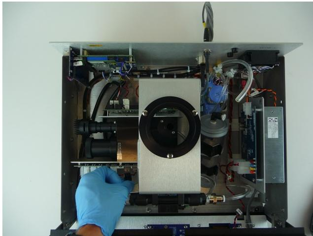
9. Close instrument and turn power on. Wait until the LED temperature stabilizes, and then perform a PMT sensor check with the SpanDust™ (Section 4.5).
