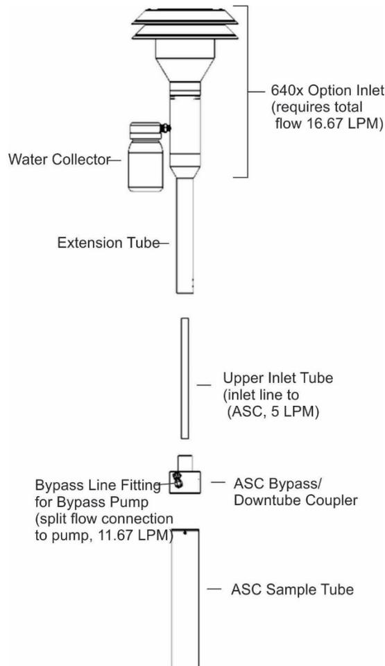
**Figure 2-14. 640X Option Inlet and ASC Assembly**
