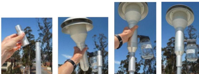
**Figure 2-19. 640x Inlet and Sample Line Assembly**
