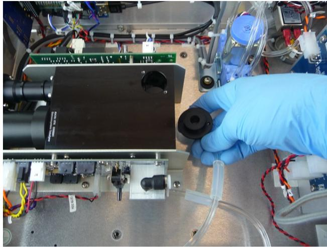
5. Clean the optics chamber interior surfaces, ensuring to include windows, with a lint-free cloth.
