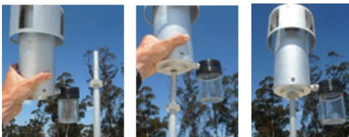
Figure 2-18. T640 Inlet and Sample Line Assembly
