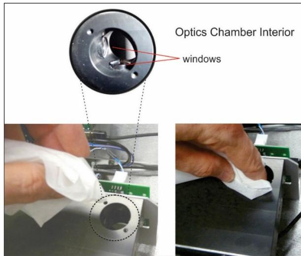
**Figure 5-6. Maintenance: Optics Chamber Windows**
