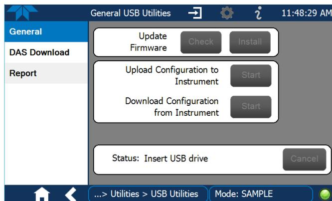
**Figure 3-8. Configuration Transfer**
