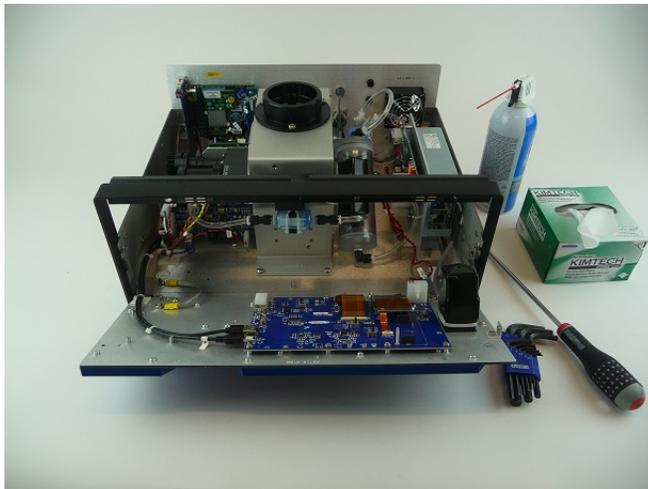
2. Remove the ASC support, which straddles the sensors.
