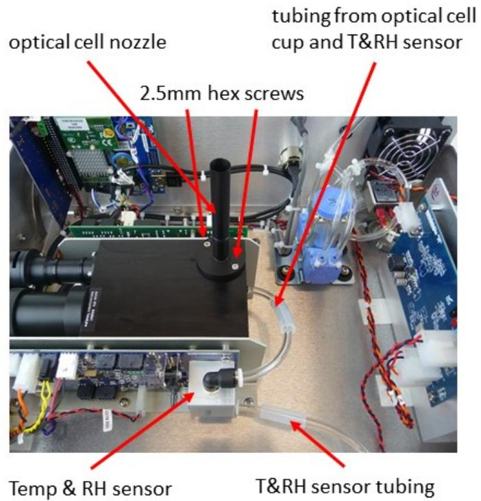
4. Remove optical cell nozzle from optics chamber, and remove cup, including its tubing, from optics chamber bottom; detach RH/T sensor tubing from the cup.
