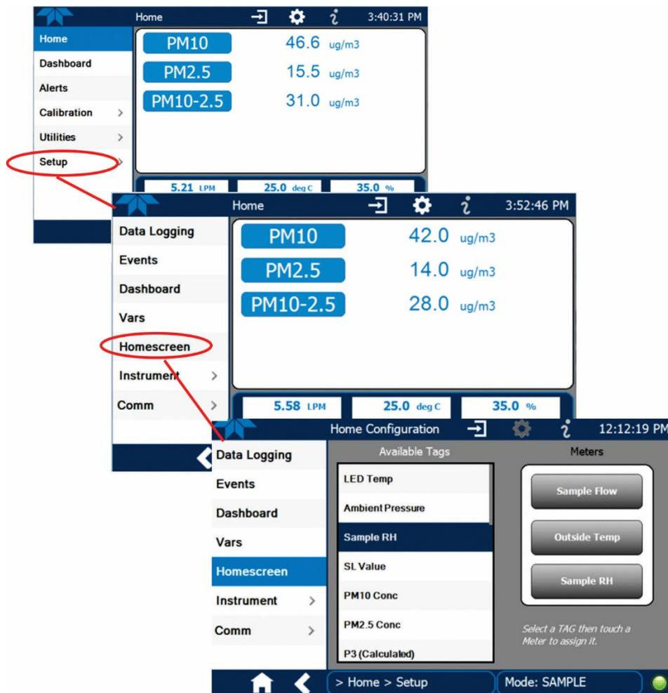
Figure 3-21. Home Configuration thru Setup Menu
