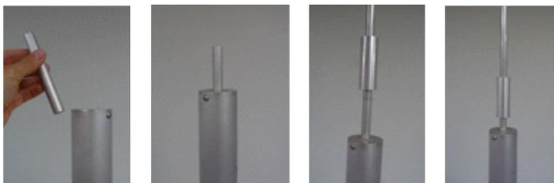
**Figure 2-16. T640 Inlet Tube and Slip Coupler Assembly**
