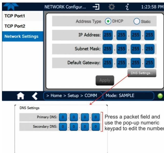
Figure 3-23. Communications Configuration, Network Settings
