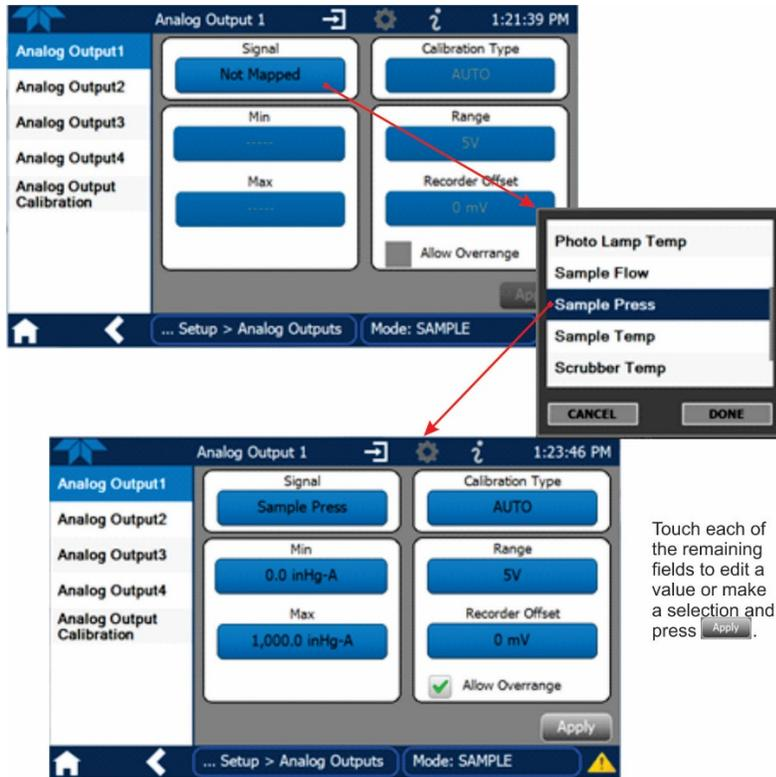
Figure 3-30. Analog Output Configuration Example
